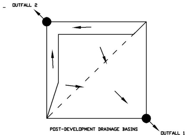
The post-development discharges for Outfall 2 are 3, 6, and 9 cfs for the 2-, 10-, and 100-year design storms, respectively. Outfall 2 meets the peak discharge requirements of the Ordinance because the post-development peak discharges are below the pre-development discharges for Outfall 2.
